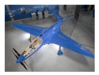
In 1938 Ettore Bugatti began to design an airplane to compete in the 1939 Italian cup races. Mostly made of wood construction the Bugatti 100 features forward-swept wings, an automatic flap system, a v-shaped tailplane with mixed controls, retractible landing gear, and two 450 HP Bugatti 50B engines, internally mounted behind the pilot, geared to drive two counter-rotating propellers. It is expected to reach 500-550 MPH.
