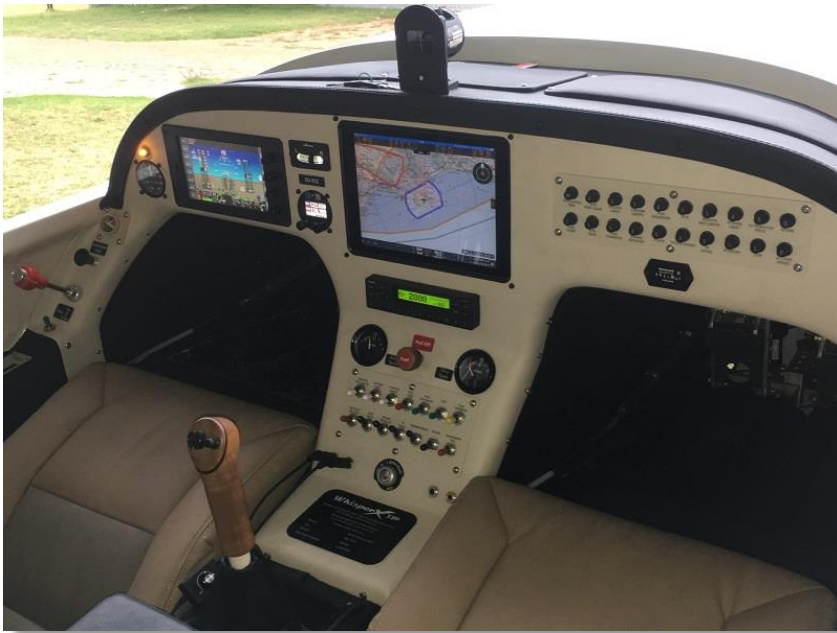
Clean cockpit layout and local Hard Pear control grip
