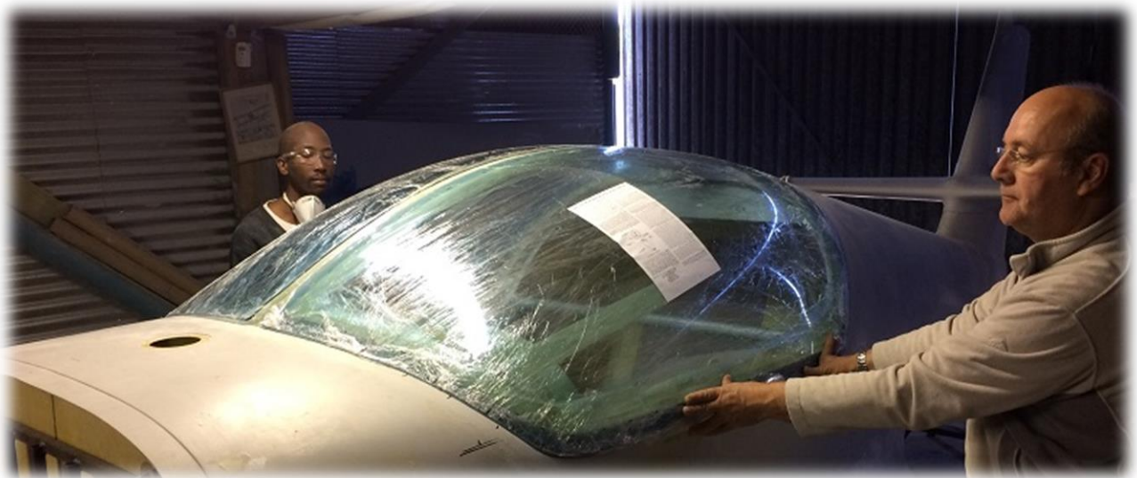
Andrias & Brett checking the canopy final fitting
