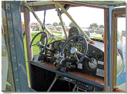
Cabin detail showing the unusual twin "steering wheel" controls jutting out from the instrument panel
