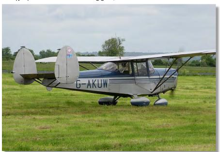
the rear fuselage. A fuselage stretch of 8.5 in improved the legroom and, combined with the accessible rear fuselage, provided a more flexible internal space. It was powered by a 155 hp Blackburn Cirrus Major 3 engine.
