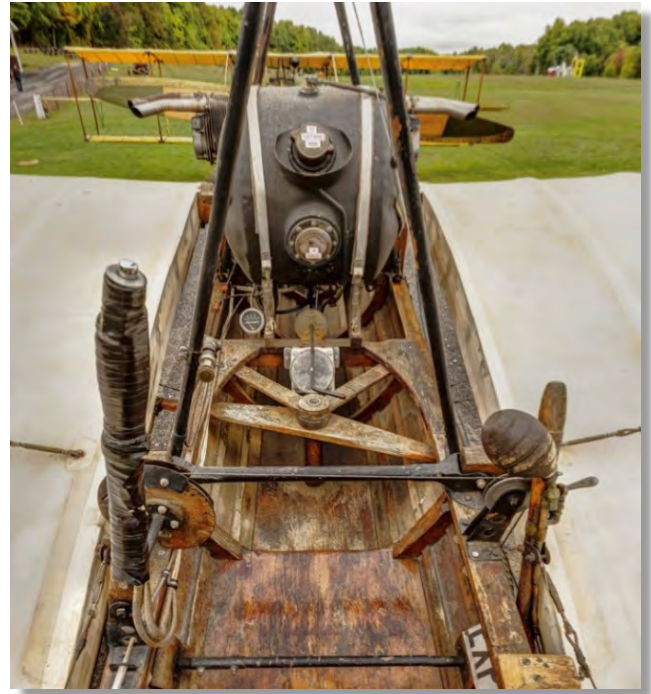
1910 Hanriot. Note the wing warping controls
