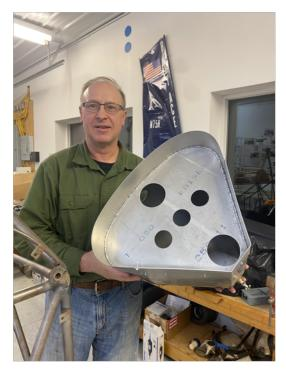
Tyler Mullen visited us during his Spring Break from Purdue. He dove right in and tied down the aluminum base on the turtledeck for the headrest fairing. We started a several week process of hand-priming the rear fuselage to prevent any more surface rusting. Longerons for the sides of the fuselage are being measured for new aluminum ones to replace the original wooden ones.
