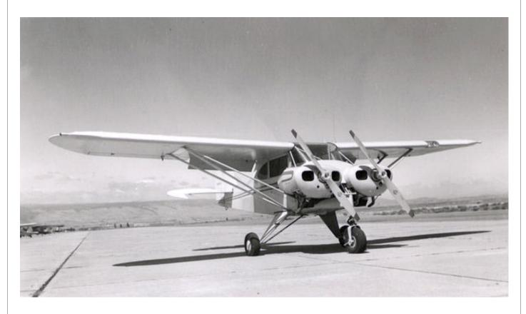
Also known as the Wagner Twin 2, Wagner Twin Tri-Pacer, and Wagner Pacer 125, this was a standard PA-22 fitted with two 125 hp Lycoming O-290-D engines mounted side-by-side. The conversion was produced in three weeks by Harold Wagner from Portland, Oregon. To clear the two overlapping propellers the left engine shaft was fitted with a 4.75 in (121 mm) extension. After 100 hours testing, the aircraft was converted back to its original configuration.
