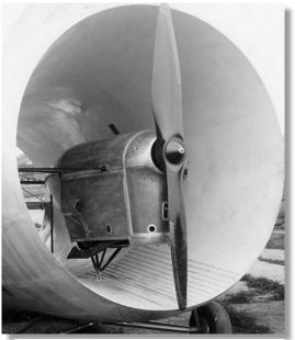
120 hp de Havilland Gipsy III inverted in-line piston engine
