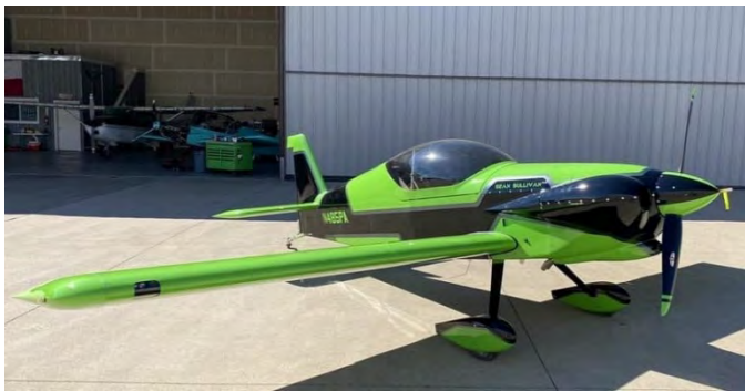
This example is covered in Vinyl Wrap and powered by a Lycoming O-235
