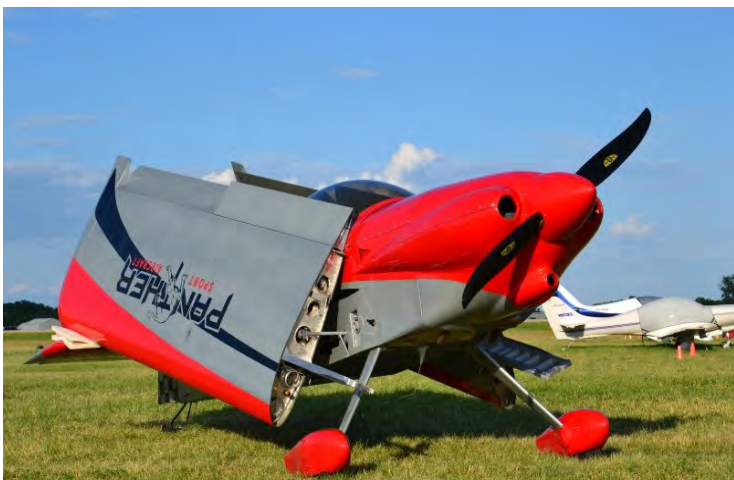
The Wings can be folded allowing hanger sharing or trailering home
