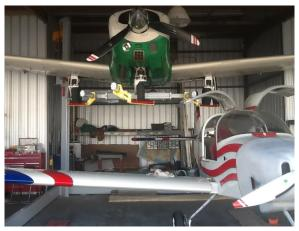
This is a 2,500 lb. capacity electrically operated hoist purchased new from manufacturer (ARM Aerospace) in 2015 and it is in "like new" condition. The lift is equipped for a nose wheel aircraft and tail wheel kits are available from the manufacturer. Asking \$8,000 or best offer. Email for more info: eagerlee6@gmail.com
