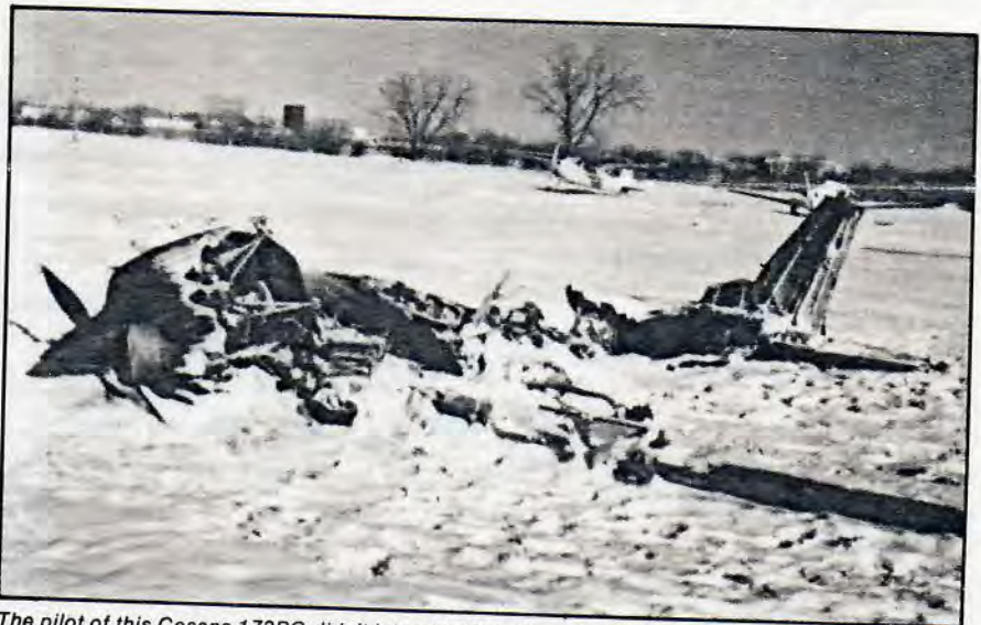
The pilot of this Cessna 172RG didn't intend to literally preheat his airplane for winter start. Improper preheating can cause major engine damage and, as shown here, can result in far more disastrous consequences.
