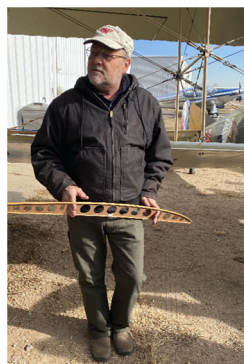
Mike Guegler with a floppy Spad wing rib, with some of the Spad struts and wires in the background.
