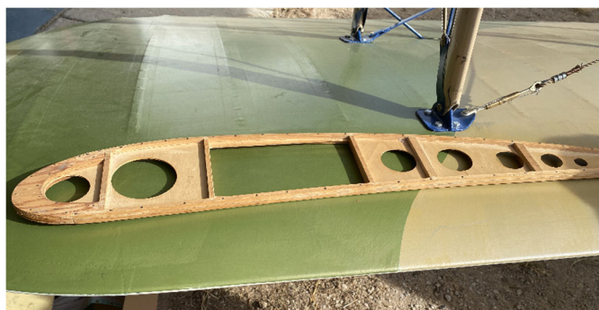
In contrast, a Fokker cantilevered wing rib
