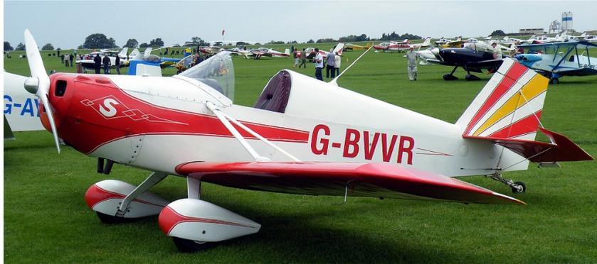
Above is an example picture of the single seat low *folding* wing aircraft in flying condition.
