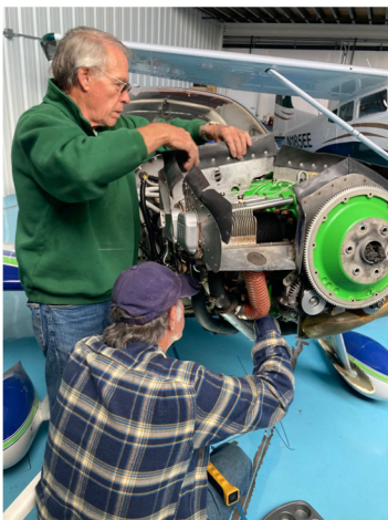
Scott Serani and Cliff Goldstein install cooling baffles in Stephanie Wells's RV-7.
