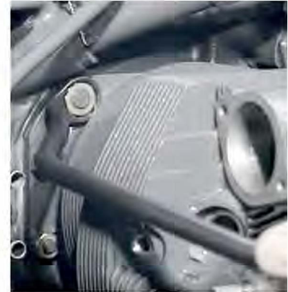
TIGHTENING A CYLINDER hold-down nut is an extraordinarily critical task. Failure to do it exactly right can result in catastrophic engine failure.
