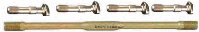
THE REDUCED-DIAMETER shanks of Lycoming connecting rod and crankcase through bolts make them less stiff and therefore their joints harder.
