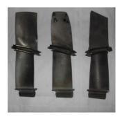
One was about the General and Electric CJ-610 CF-700 Turbo Jet Engine. These two engines are nearly the same except the CF-700 which has an radial air bypass and has a different combination turbine blade (as shown at the bottom picture,) in the and compressor blade(as shown at the top). The CJ-610 is rated at 3000 pounds of thrust and the
