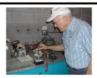
picture of Frank in this space. Frank and I gave a program, not so long ago, discussing the techniques in servicing engine spark plugs. Here, Frank is demonstrating a resistance in an aircraft Spark Plug. Often times the resistance goes up and produces poor engine performance.
