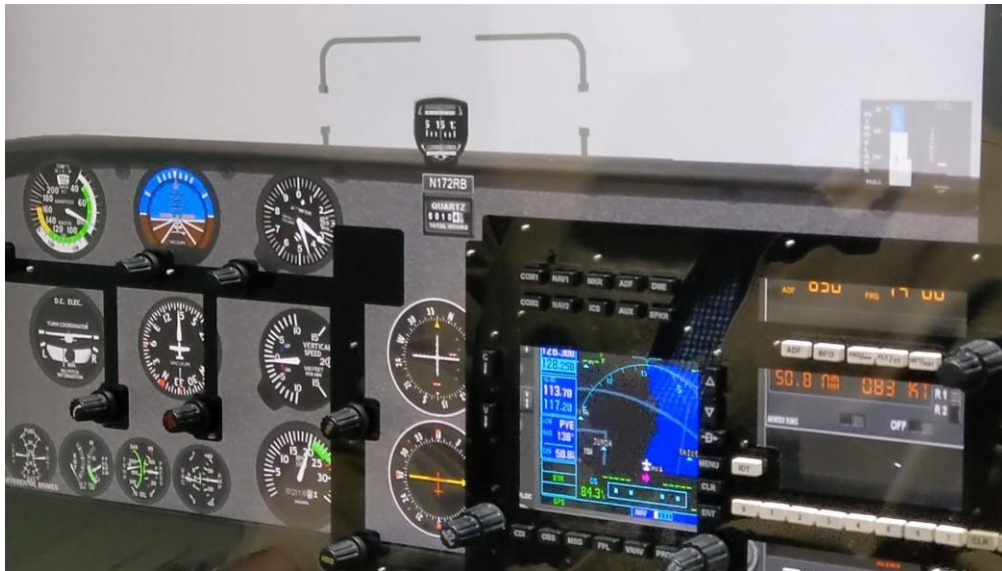
Closeup of steam gauge panel with Garmin 530 nav/com radio. Note knobs on panel to adjust instruments and radio.
