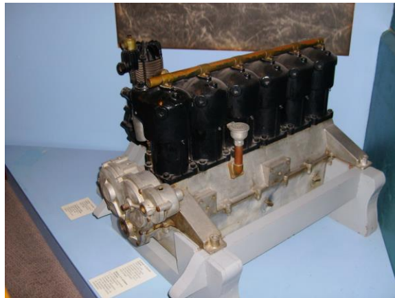
Curtiss engine used for the first Canadian built aircraft
