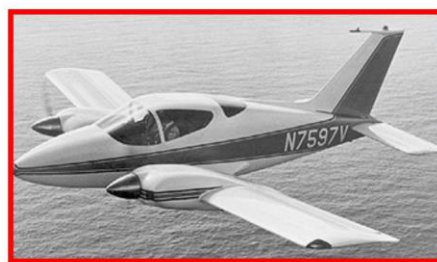
Wing Derringer— Designed by John Thorp. Max speed 231mph Range 626mi. First flew 1964, 12 built between 1964 and 1982
