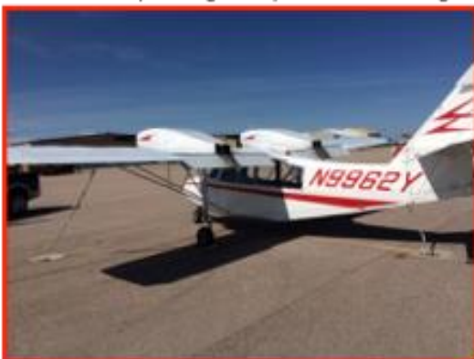
No fabric on this airframe—factory fiberglass covering
