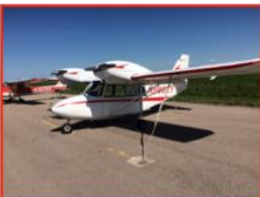
Engine/prop placement make for a noisy front seat and greatly reduced visibility for the pilot when turning.
