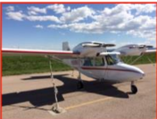
Engine/prop placement make for a noisy front seat and greatly reduced visibility for the pilot when turning.
