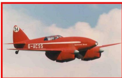
deHavilland DH.88 Comet Racer— Designed for the 1934 MacRobertson Air Race. Max speed 237mph, Range 2925mi.
