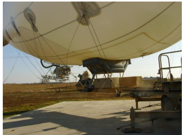
Instrument package on structure under the balloon. Can be radar, camera, or scientific instruments to customer's specifications
