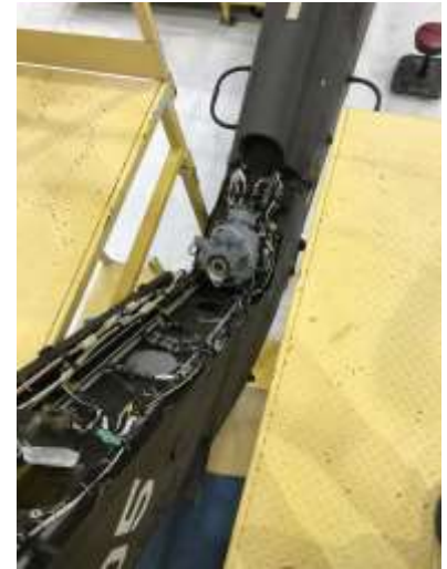
A closer view with the both drive shafts removed for inspection.
