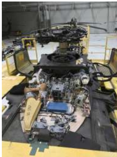
The very complex control area forward of the rotor hub. Once disassembled for inspections, the procedure to reassemble and rig each control is quite exact and time consuming.
