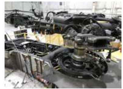
The rotor hub with the dampers, and other control components along with the washplate are shown here.
