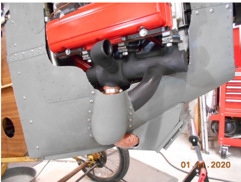
19. Current Stage, Exhaust Fabricated, 1/11/2020
