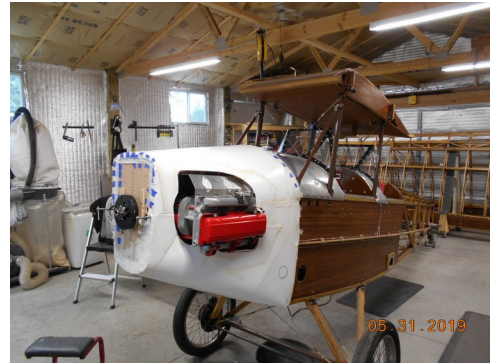
7. The Cowling Fabrication Stage, 5.31.2019
