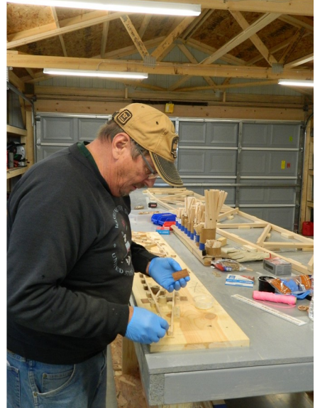
2. Made a jig, started gluing all the sticks together 4.30.2017r
