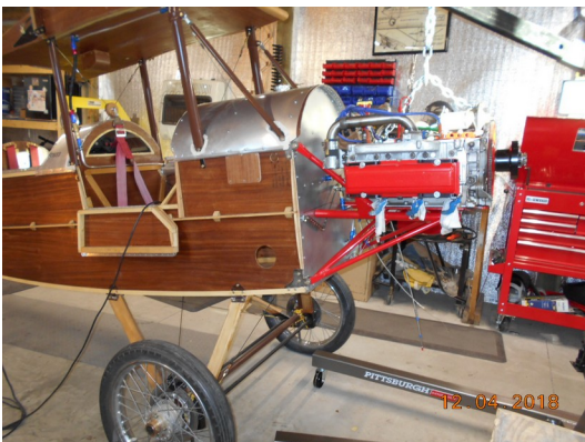
E5. engine Mount Fabricated and Secured 10.2.2018
