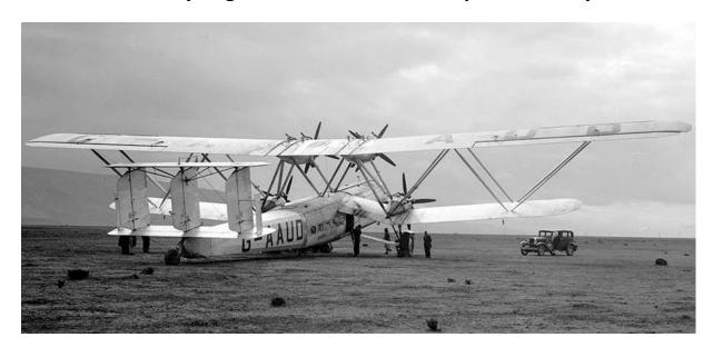
The Handley Page H.P. 42 was the world's first four-engined aircraft. It was also the largest at the time. The H.P. 42 made its first flight on November 17 1930. A total of eight aircrafts were built for the new Imperial Airways. For more>>
