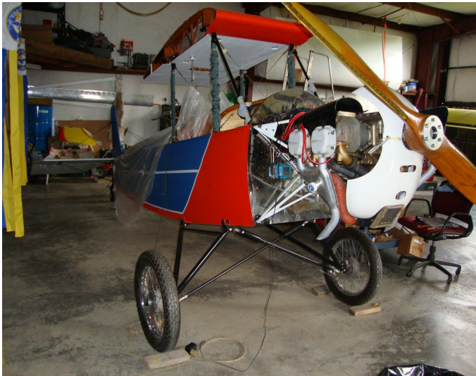
The cowling being fabricated (the white nose bowl)
