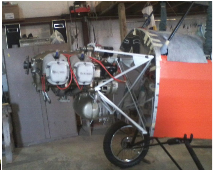
The engine installed and the engine mount we fabricated
