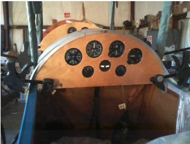
The instrument panels that we fabricated being fitted
