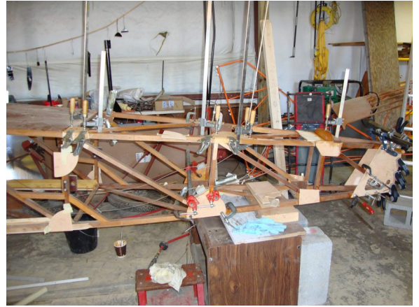
The gussets being fitted and glued on
