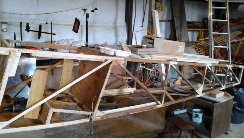
Fuselage stripped and ready to start adding the plywood gussets
