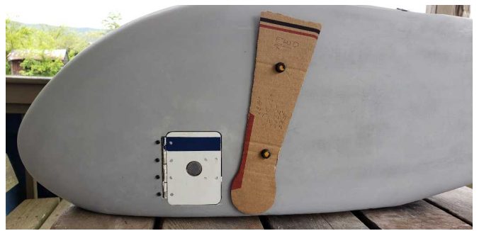
Stripped & filled hole to replace with an access door from an old wheel pant.
