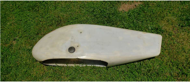
Stripped & filled hole to replace with an access door from an old wheel pant.
