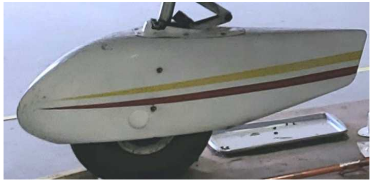
Old beat up & cap & hole to access tire fill valve.
