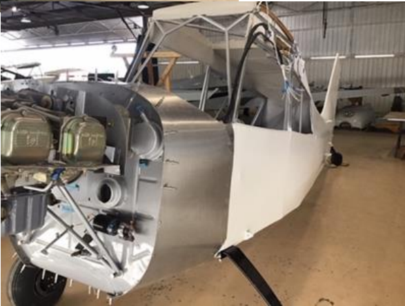
Photo 15: New boot cowl being fitted.
