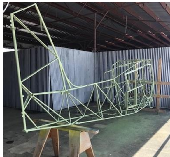
Photo 5: Epoxy on fuselage.
