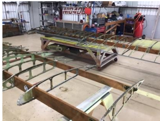
Photo 18: Wings being repaired.
