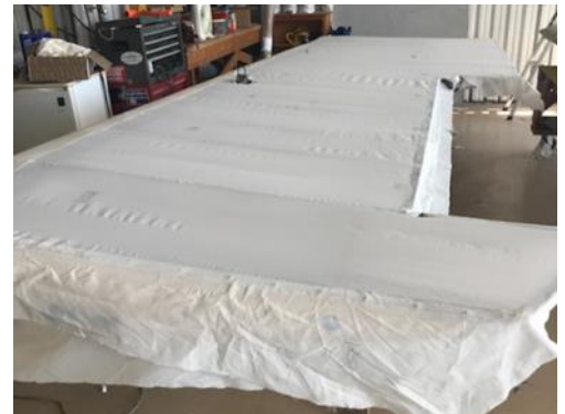
Photo 19: Wings getting covered. Glued on and being shrunk.
