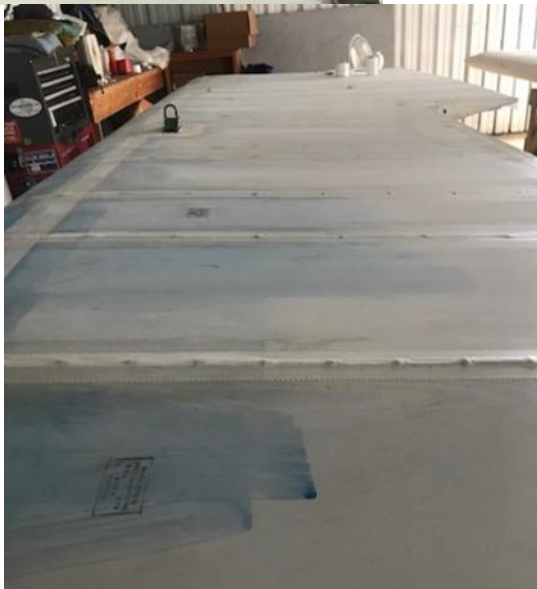
Photo 21: Finishing tapes are going on. Nitrate dope is already on. We switched from tinted to non-tinted nitrate due to availability. Lead time on the dope was dictated by Covid.
