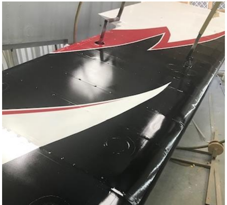
Photo 23: Wing is in a turning fixture making final livery much easier to apply.
