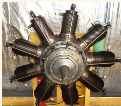
A 100 hp Gnome 9-B2 rotary aircraft engine,
