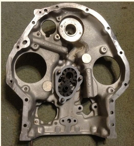
Inside of Lycoming Accessory Case Showing Oil Pump
