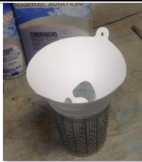
Photo 6: Paint strainers are a must. You can't blow chunks through a spray gun.
