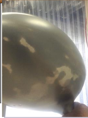
Photo 5: The same wheel pant held up to bright light. Green primer makes the silver look like silver-green. Places where the primer was sanded through or too thin let light pass. In the bright sun this will probably look like a mottled finish.
