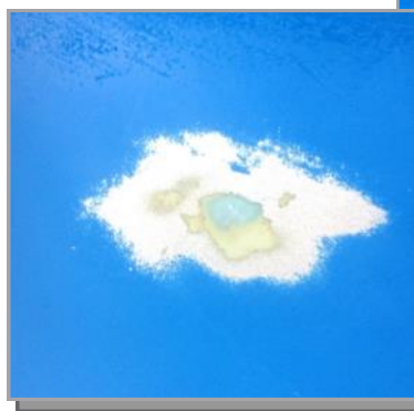
Photo 3: When a low spot is really more like a crater, spot putty is used to fill the hole. Spot putty sands easily. Color compatibility is also important for the spot putty unless you want a measles finish.
