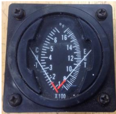
Photo 3: Dual voltmeter calibrated for J and K thermocouples
