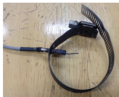
Photo 2: Type K thermocouple (EGT) with the protective sheath burned away
