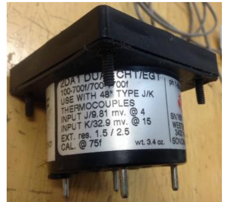
Photo 4: Here is the label on the CHT/EGT indicator showing temperature range and
