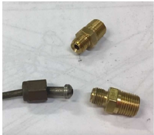
Photo 2: Primer nozzle with the copper fuel line disconnected.
