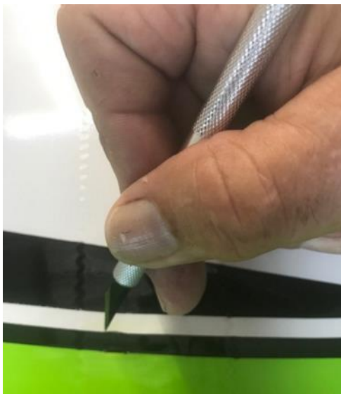
Photo 5: Scrape off under spray. This photo is a bit misleading. Use the edge of the blade for scraping not the tip
