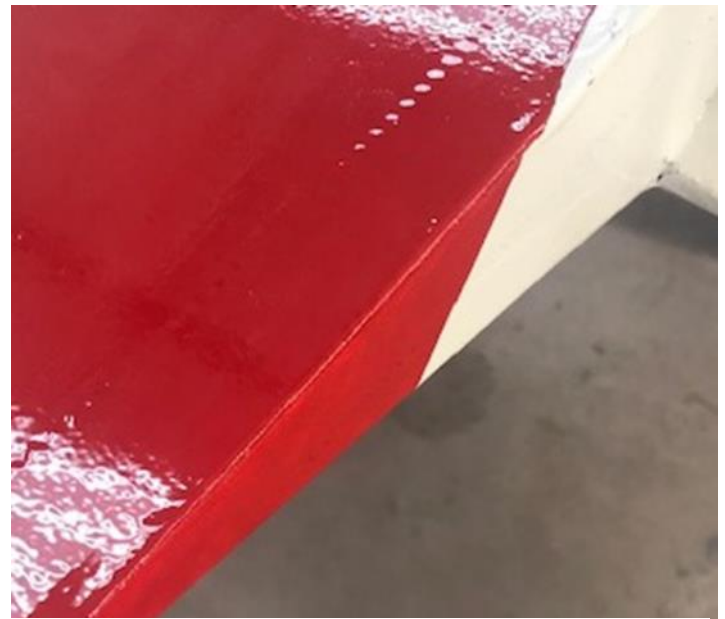
Photo 10: Touched up aileron cove. The red top surface of this wing was easy to shoot but going over the corner and into the aileron cove was much easier to do with an airbrush afterwards. A lot depends on how complicated the paint scheme happens to be.
