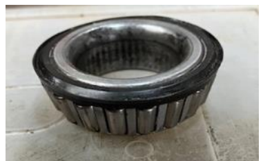
Photo 3 and 4: Bearings with molded-on seal.
