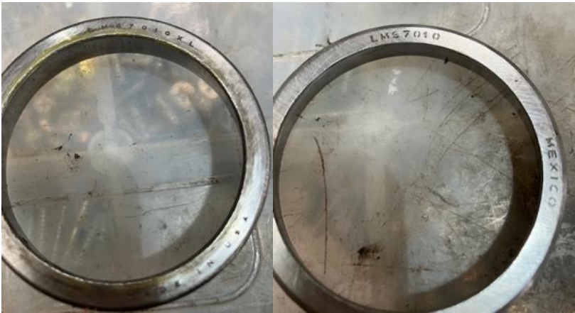
Photo 5: Correct cup for the Goodyear wheel. p/n 7010XL
