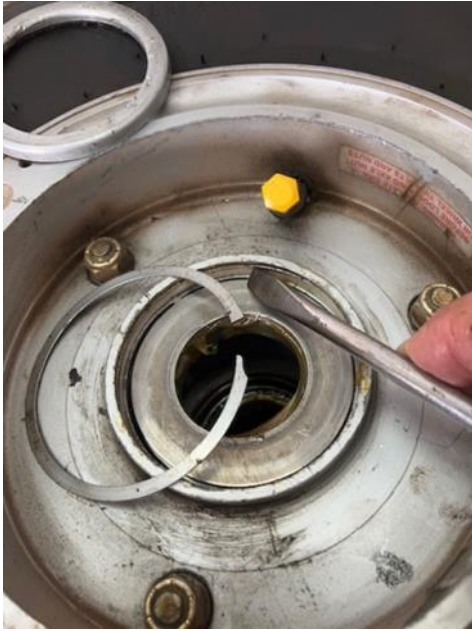
Photo 1: Screwdriver pointing to groove for the snap ring.
