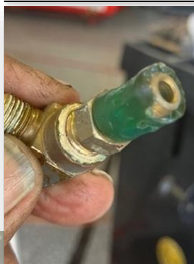
Photo 10: Please DON'T use box store tubing for fuel. This homebuilt was almost a flaming streamer. The green tube disintegrated after being lightly wiggled during an inspection.
