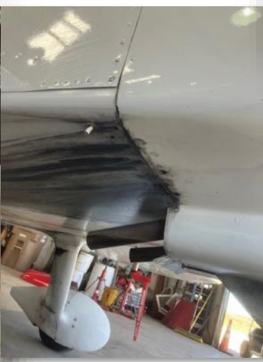
Photo 7: Owner said he had an oil leak. Sure enough, the nose seal had blown out. Just kept flying, adding oil and waited for the annual.
