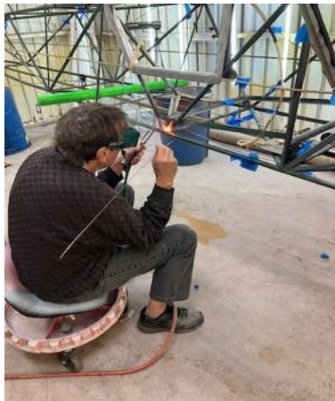
Photo 5: Welding. Note blue tapes to mark holes.
