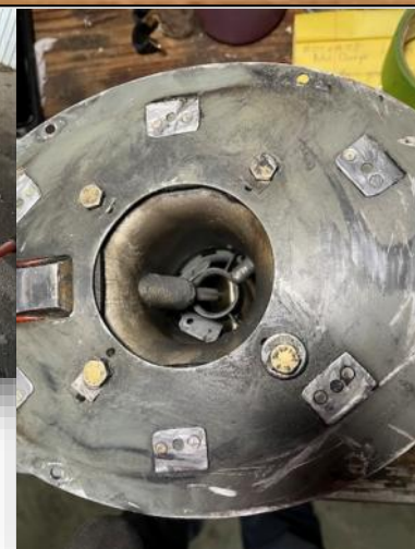
Photo 9: Owner reported weak performance. Broken intake pieces are lodged in the updraft carburetor of this RV homebuilt.
