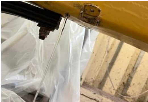
Photo 1: Water pouring out of longeron.
