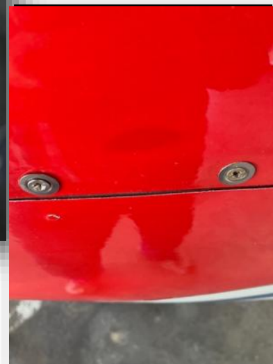
Photo 11: Sharp eyes? One of these screws is a 90-degree countersink from the hardware store and one is an aviation screw with 100-degree countersink.
