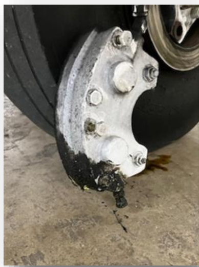
Photo 6: How good is your pre-flight? This brake caliper is screaming, "Leaking O-Rings."
