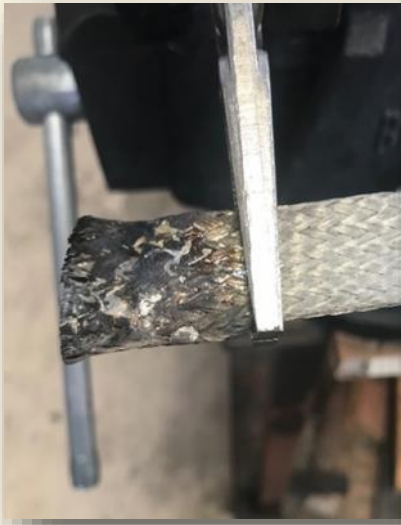
Photo 3: Soldered braid. Soot can be gently cleaned off with a wire brush or light
