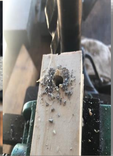
Photo 4: Wood-metal sandwich. Clamp well and drill slowly.
