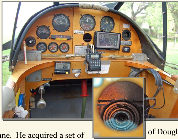
The fuel sight window is visible through a hole in the panel
