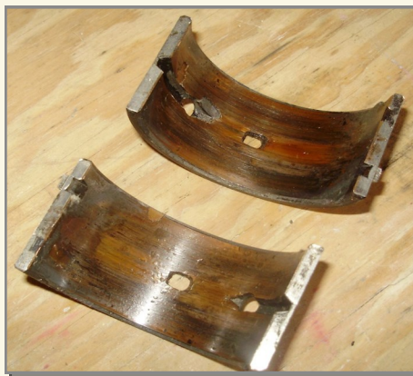
Worn Out Center Main Bearing of Lycoming O-320
