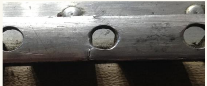
Photo 3: A cracked Cessna seat rail.
