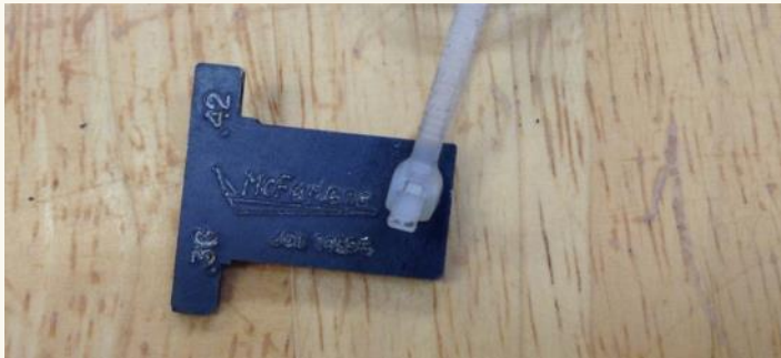
Photo 2: McFarlane Seat Rail Wear Gauge. Early version has .36 and .42 measurement. Current gauge only has .42 which is all that is necessary.
