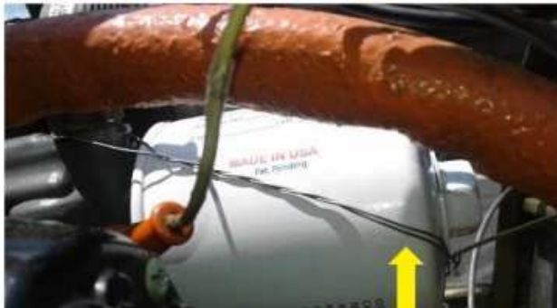
This oil filter was not properly safety wired. The wire is routed in the right direction, but there are too few twists per inch. The arrow points to the section with no twist.
