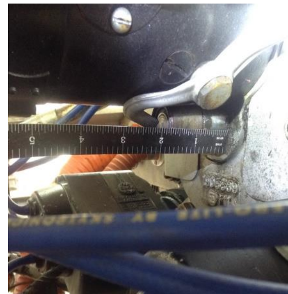
Photo 3: Measuring travel of the starter shaft.
