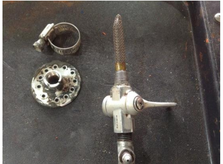
Photo 5: Cracked fuel bung and fuel valve disassembled.
