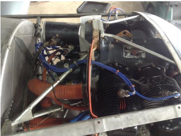
Photo 1: Starter at upper left is actuated by pulling a T-handle in the cockpit.
