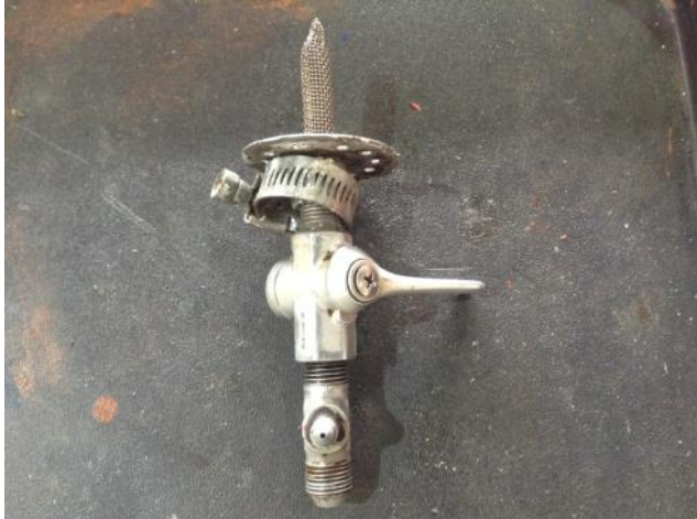
Photo 4: Fuel outlet and fuel shutoff valve.
