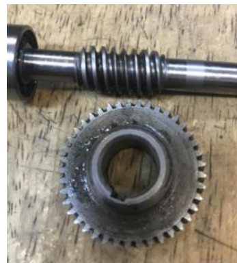
Photo 2: Gears removed from Duke's gear retract transmission.
