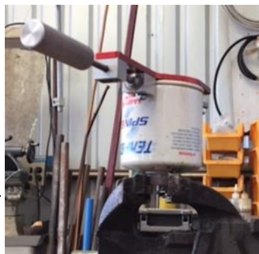
Photo 3: Filter cutter on top of an oil filter.
