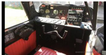
Front cockpit (the controls on the left are for trim, not engine controls)
