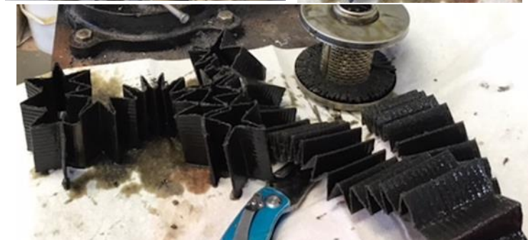
Photos 6, 7 & 8: Cutting off the pleated filter element.
