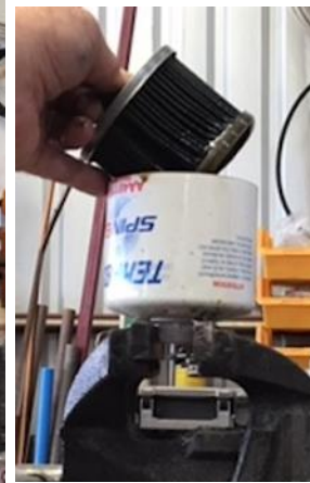
Photo 5: Remove the pleated filter element.
