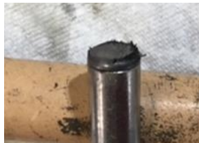
Photo 14: A small amount of iron filings on the magnet. No problem here.
