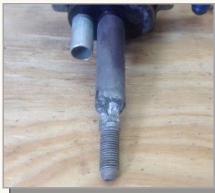
Photo 6: This gascolator standpipe is badly corroded.
