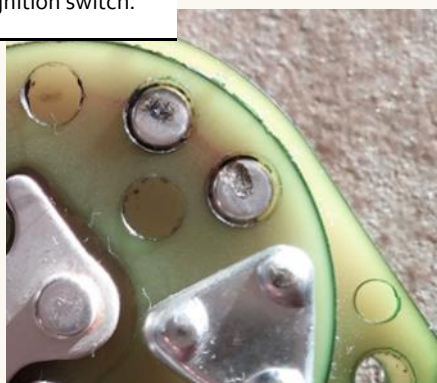
Photo 2: Here, the contact points are cleaned. Look at how much metal is eroded from some of the contacts! Photo credit: Vic White
