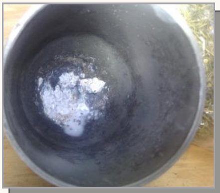
Photo 5: Chunks of hard aluminum oxide a gascolator bowl.
