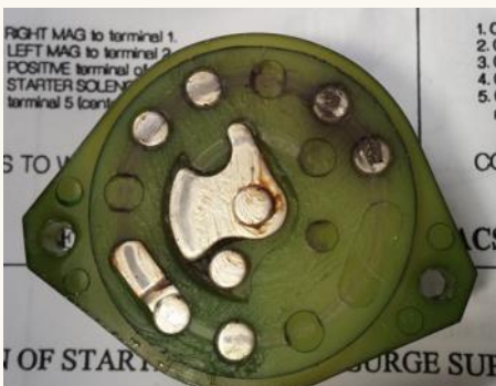
Photo 1: Inside a burned ignition switch.
