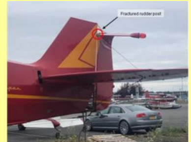
Figure 2. Photograph showing the fractured rudder post on N4206H (case number ANC21LA064).
