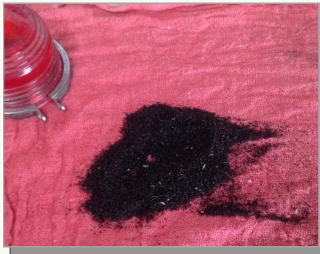
Photo 2: Trash removed from fuel strainer. This is about ¼ of the quantity removed.
