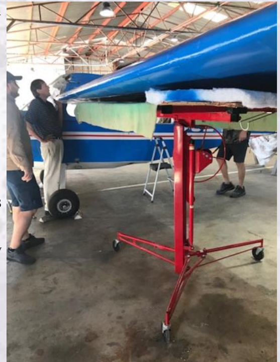
Photo 3: Wing being raised and guided into position
