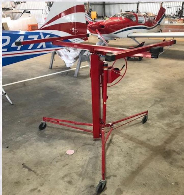
Photo 2: Sheet Rock Hoist
