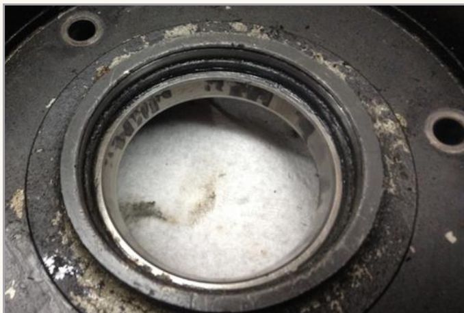
Photo 1: Bearing race is corroded.
