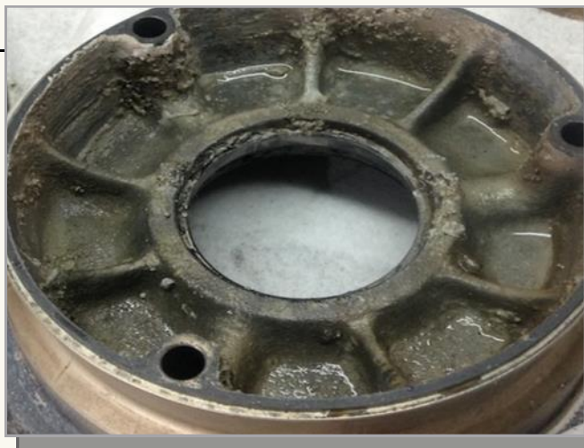
Photo 2: Water and corrosion inside the wheel.
