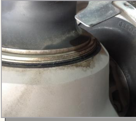
Photo 5: Propeller showing signs that an overhaul is in the near future.
