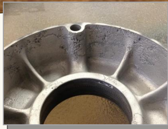
Photo 3: The magnesium is pitted.
