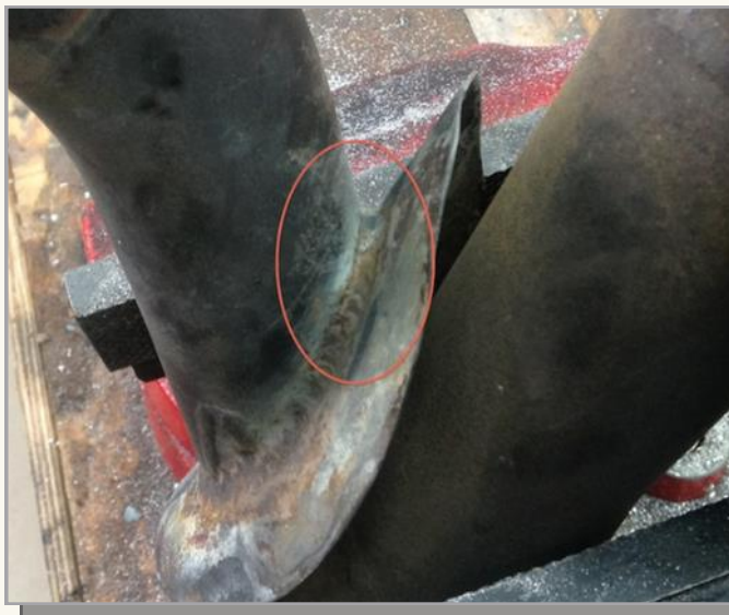
Photo 4: Exhaust header in a vice. Telltale gray soot shows exhaust leak.
