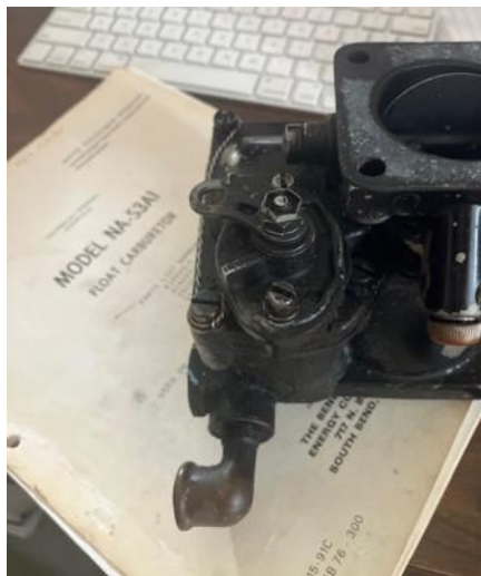
Photo 2: NA-S overhaul manual and a very dirty NA-S carburetor. The difference between the NA-S2 and NA-S3 is that the S3 mixture control was optional.
