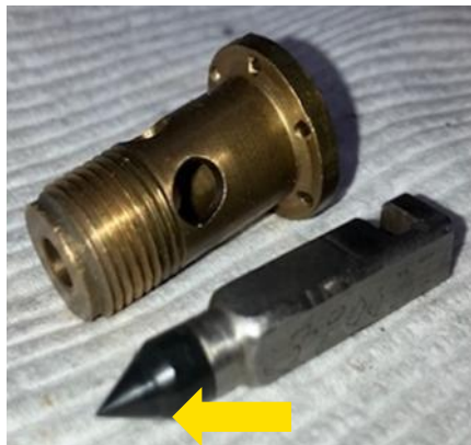
Photo 6: An old neoprene needle and its seat. The groove in the tip of this needle is not good.
