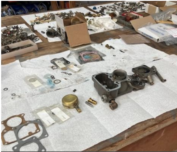
Photo 12: Stromberg NA laid out for repair and the author's spare parts stash
