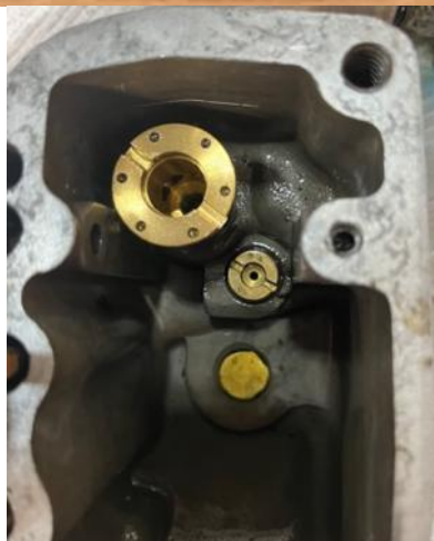
Photo 7: A float bowl with the float and needle removed. The needle seat is the large brass fitting. The metering jet is the smaller, slotted brass fitting with the hole in it. It is stamped "50" meaning that the orifice is a drill size 50. The last brass fitting is a drain plug. Fuel enters through the seat and exits through the metering jet.
