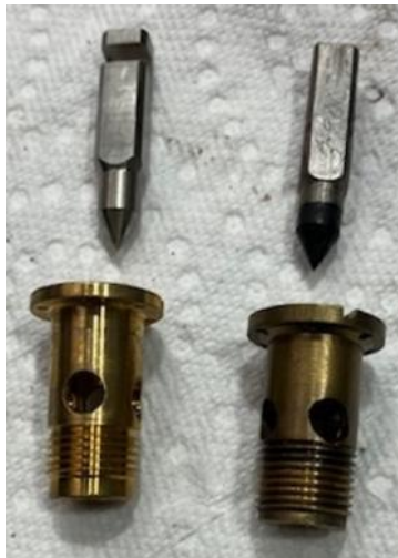
Photo 10: New steel needle and old neoprene needle.
