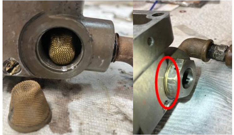
Photo 4: Large nut that holds the fuel strainer in place. Note the brass washer.
