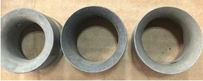
Photo 9: Different size venturis that can be inserted into an NA-S carburetor.
