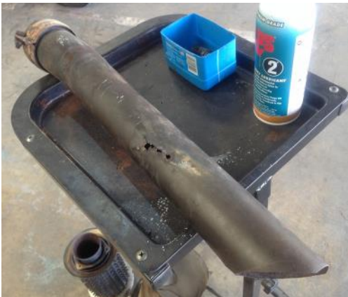
Photo 2: Tail pipe from the same Bonanza. Both sides of this tube are burned through.
