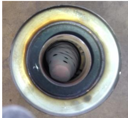
Photo 1: Sagging flame cone in a Bonanza muffler
