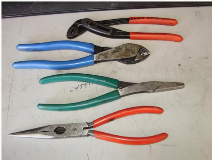
Compact water pump pliers, side cutters, duckbill, and needle nose pliers.
