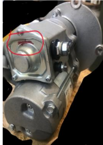
Photo 3: A starter for an older Continental engine. The configuration is different. There ought to be spare shear pins in the red circle, but somebody already used them
