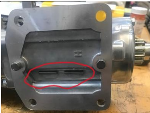
Photo 2: Underside of the same starter in Photo 1. Notice there are two spare shear pins glued to the bottom of the starter housing.
