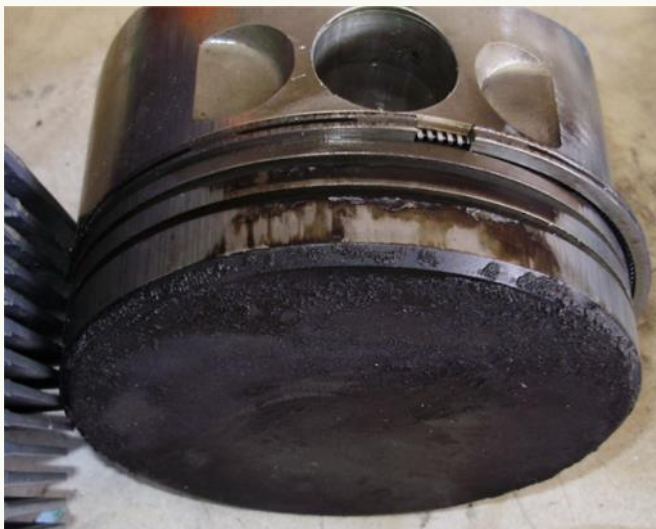
Black streaking is due to exhaust gas blowing past the rings.
