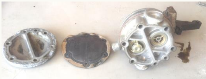
Figure 2: The bottom of the fuel pump shown disassembled.
