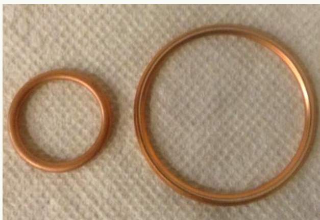
AN 900 gaskets. "Broken face" shown on right hand gasket.
