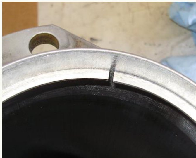
Ring Gap! Should be .02 but here it is about .125 inch.
